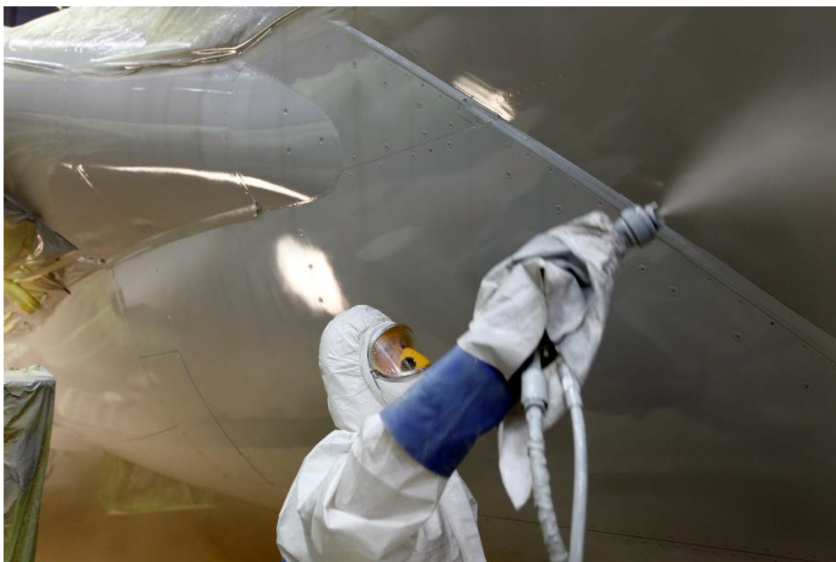
Figure 17: Application of a coating layer with a high volume low pressure (HVL) hand-held spray gun, example 2.
