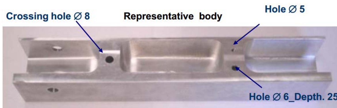
Figure 26: Representative body used in the assessment of layer thickness and heterogeneity of sol-gel coats applied by means of dip coating (Cerde, 2011)
