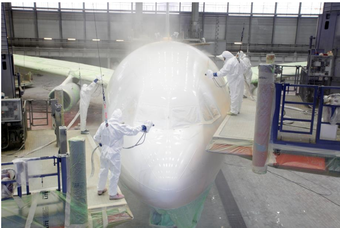
Figure 16: Application of a coating layer with a hand-held spray gun, example 1.
