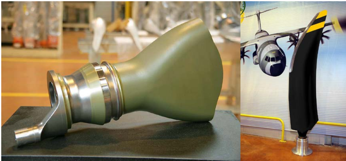
Figure 15: Bonding primer applied on the propeller tulip in green (left) which contributes to the bonding performance between the tulip and the composite blade (right). (UTC Aerospace Systems – Propeller Systems, 2014).
